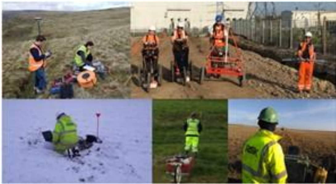
Geophysical techniques discussed from top LHC clockwise: Resistivity, Ground Penetrating Radar, EM conductivity, Seismic, Magnetics and Gravity
